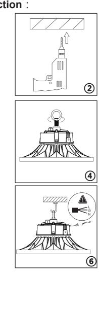
Note : The installation base must be able to support 10 times weight of the products
